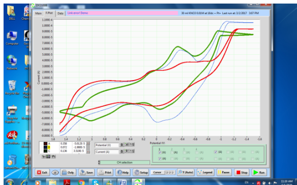
Fig. 7. Life cyclic voltammograms of medium 0.1 M KNO 3 , red, plus 0.5 ml CaCl 2 blue, plus 0.5 ml SrCl 2 green at 18 °C using Pd Electrode.
