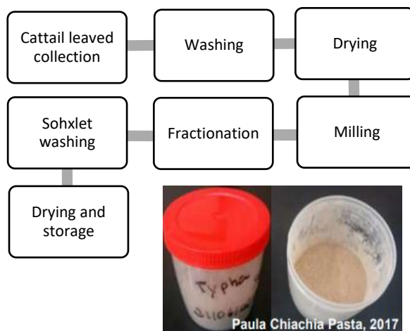
Fig. 2. Flowchart for preparing and obtaining the biosorbent. Source: Paula Chiachia Pasta, 2017.
