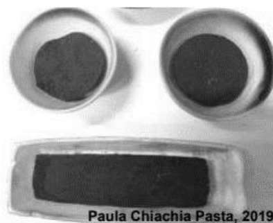
Fig. 10. Activated carbon produced after burning of the biosorbent (cattail) in muffle. Source: Authorship.
